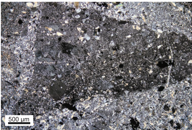
Crystal lithic tuff with silicification and sericite alteration (XPL, 5X)
