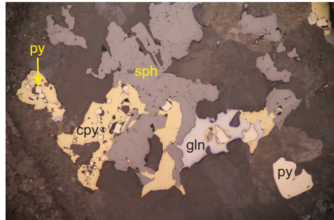
Sulfides are pyrite. locally cubic form, rimmed by chalcopyrite and sphalerite and galena (RL, 10X)
