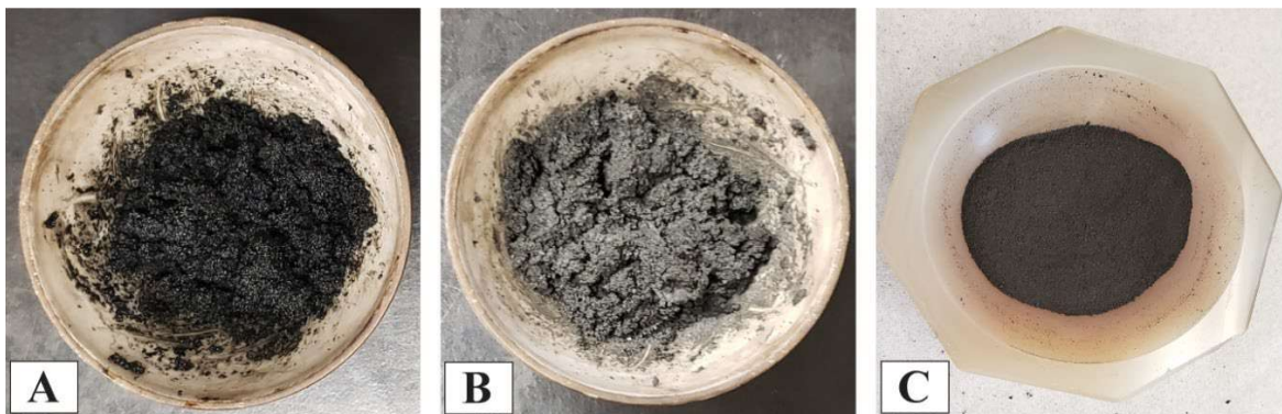
Figure 13. Photos of tailings sample before and after acid baking at 200°C using a muffle furnace: A) tailings mixed with acid, B) acid-baked tailings, and C) de-agglomerated baked tailings before water-leaching stage
