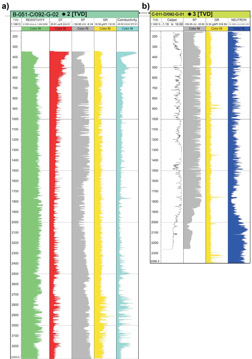
**Figure 8.** Two of the available wireline logs for wells drilled in the Lower Mainland of British Columbia: **a)** wireline log from unique well identifier B-051-C/092-G-02, and **b)** wireline log from unique well identifier C-011-D/092-G-01 (BC Oil and Gas Commission, 2022). Both logs are corrected for true vertical depth (TVD), given in metres. Abbreviations: DT, sonic log; gAPI, API gamma-ray unit; GR, gamma ray; mS/m, millisiemens per metre; mV, millivolt; SP, spontaneous potential.
