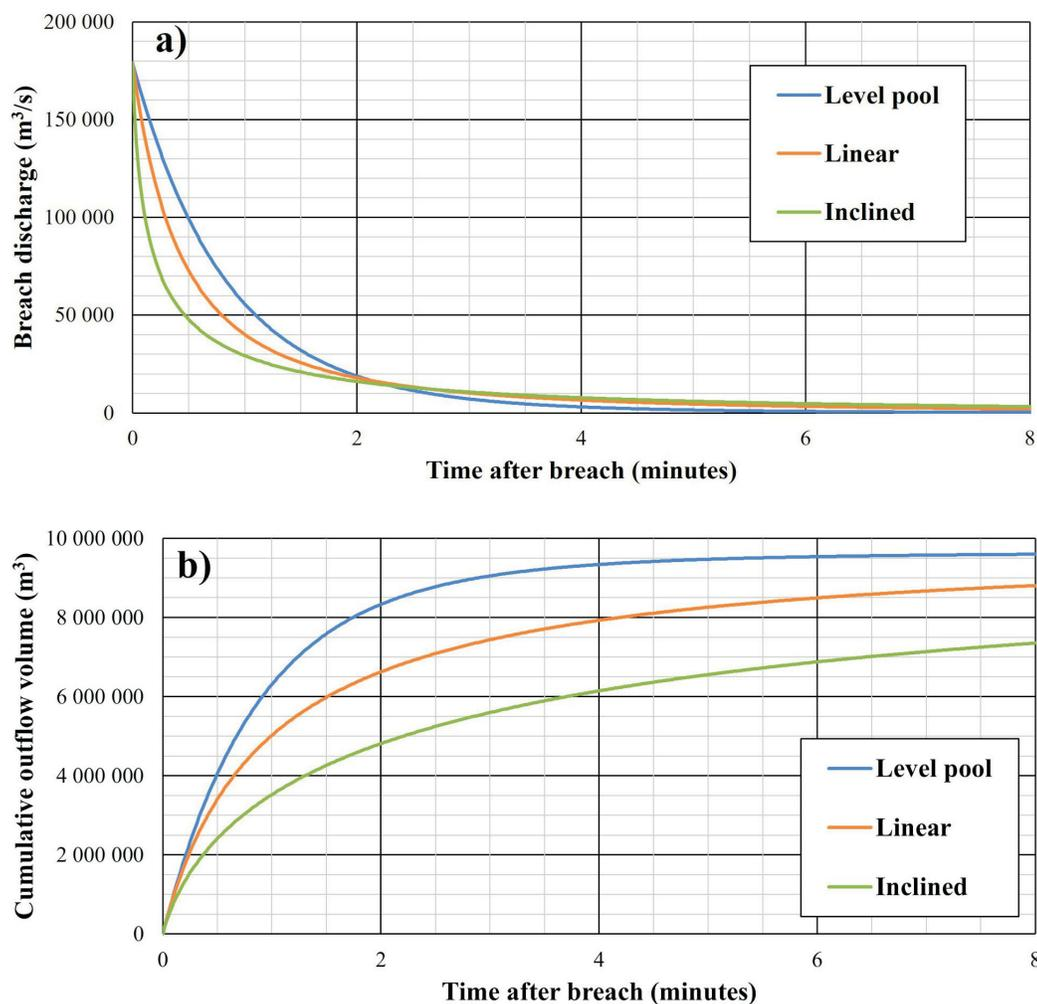
Figure 7. a) Modelled breach hydrographs. b) Cumulative outflow volumes for the Feijão event.
