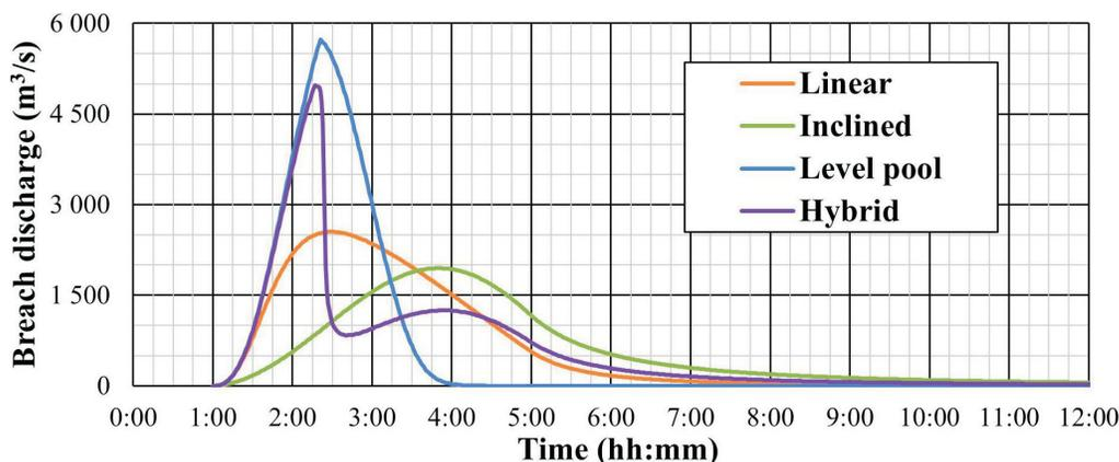
Figure 6. Modelled breach hydrograph for the Mount Polley event.
