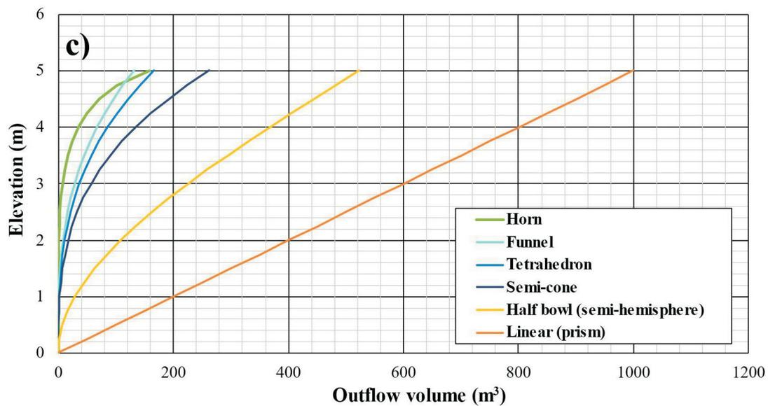
**Figure 1.** a) Six idealized shapes for the post-failure depression of tailings facilities. b) Stage-storage curves for the idealized shapes in relative values. c) Stage-storage curves for the idealized shapes in real values.
