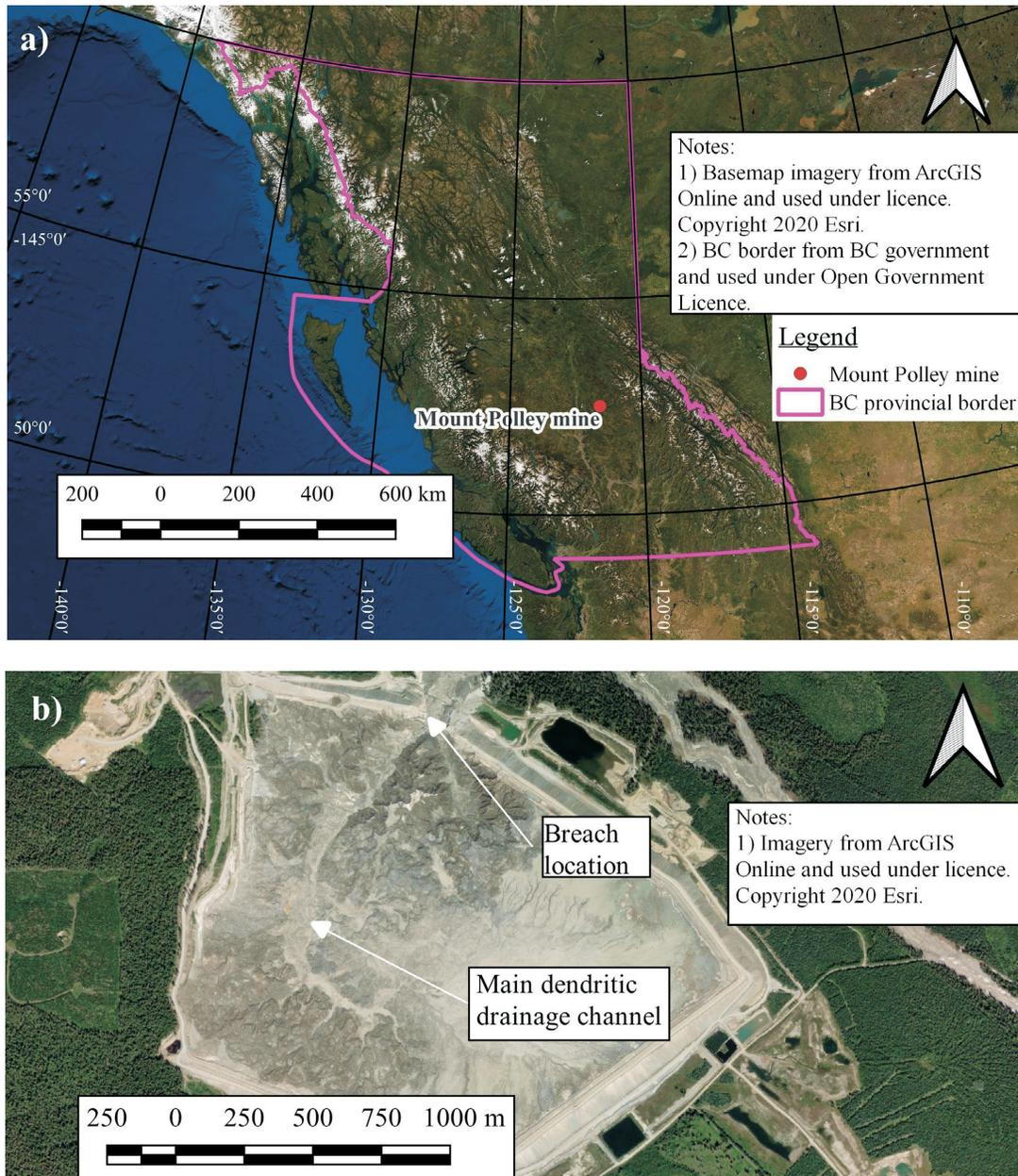
**Figure 2.** a) Location of the Mount Polley tailings-storage facility. b) Post-failure aerial imagery of the Mount Polley tailings-storage facility.
