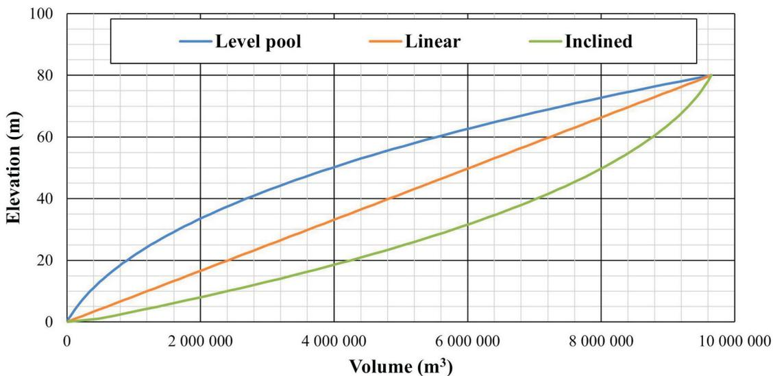
Figure 5. Estimated stage-storage curves for the released tailings in the Feijão breach event.
