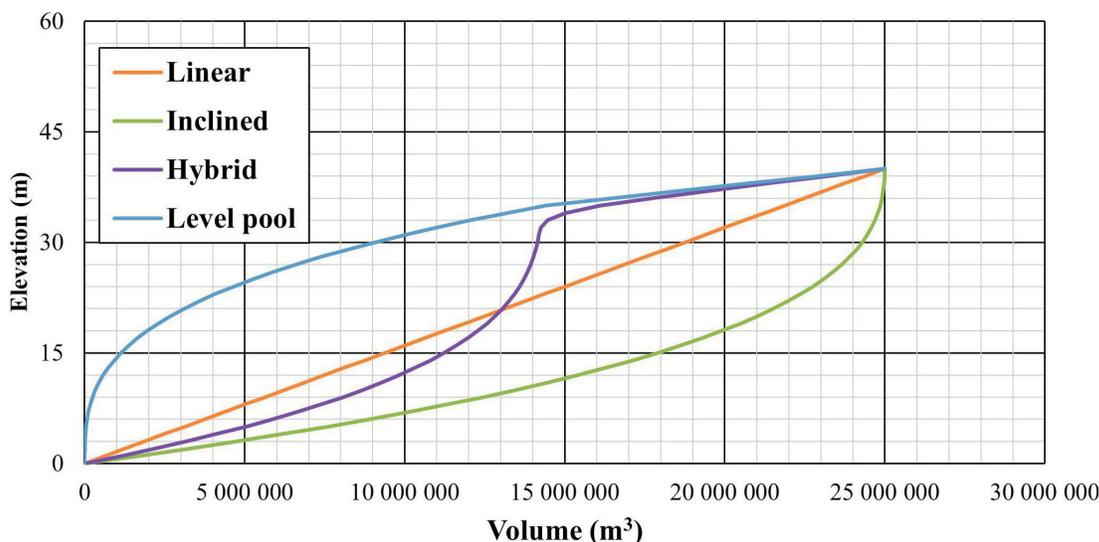
**Figure 3.** Estimated stage-storage curves for released tailings material and water in the Mount Polley breach event.
