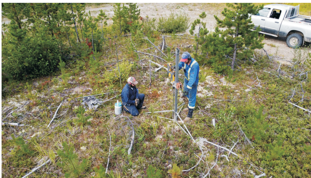
Figure 2. The Talon Drill™ system tooling with custom bits and samplers specifically designed to work within the difficult drilling conditions encountered when sampling subglacial till. This system enables the collection of high-quality till samples anywhere the till occurs at or near the surface. This method of till sampling overcomes the limitations of standard opportunistic sampling programs, which can result in suboptimal sample distributions because of the reliance on sampling existing exposures.
