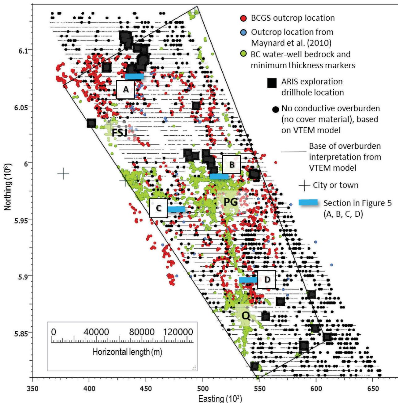
**Figure 4.** Constraining data used for overburden-thickness modelling. Constraining data from VTEM inversion models are derived from interpretations digitized along line on east-west VTEM lines spaced 4 km apart. Project area lies within the black quadrilateral. Abbreviations: PG, Prince George; FSJ, Fort St. James; Q, Quesnel.
