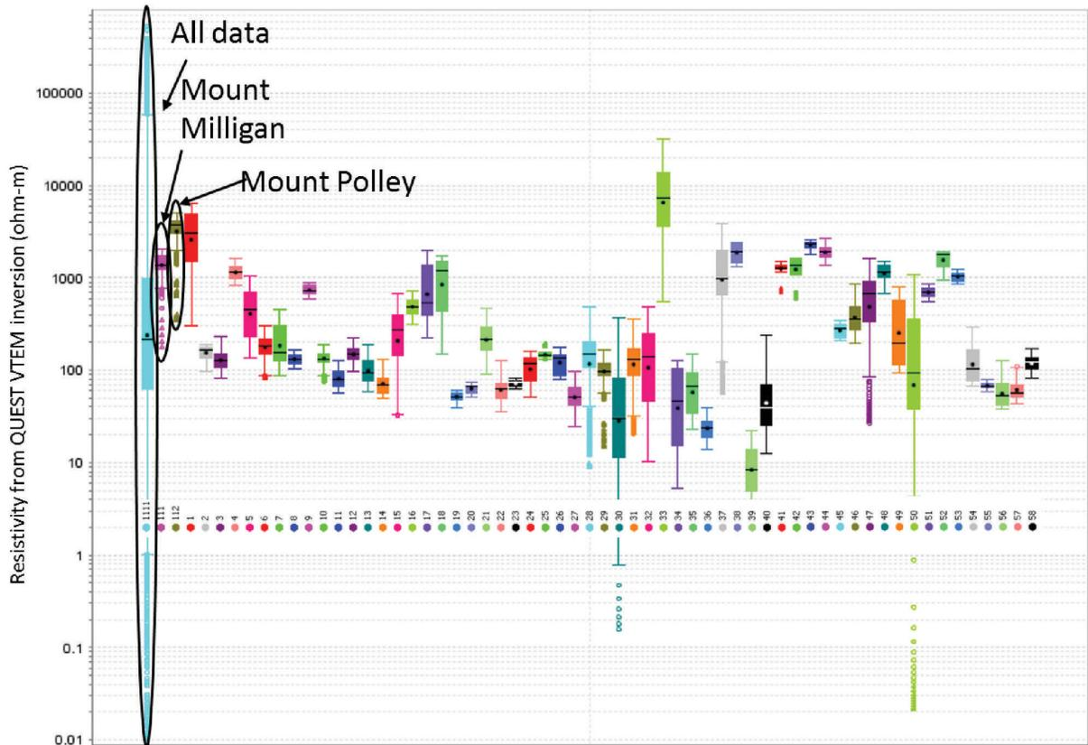
**Figure 9.** Density (upper plot) and resistivity (lower plot) ranges for each of the 58 magnetic targets (colors assigned randomly) sampled from regional gravity and VTEM inversions, compared to density and resistivity ranges for the entire QUEST project area and those associated with the Mount Milligan and Mount Polley intrusions.
