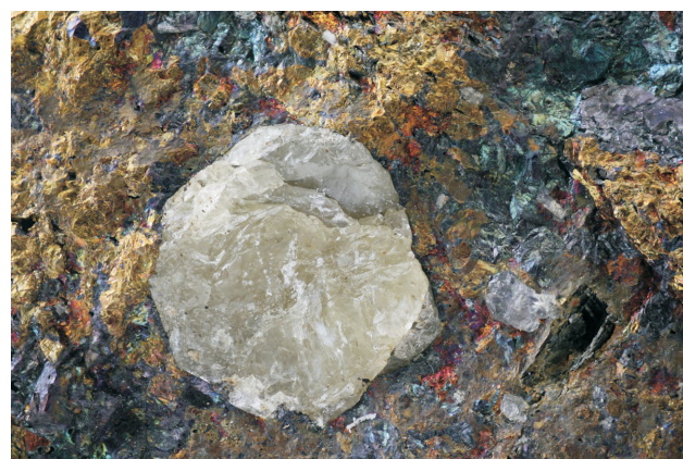
Figure 3. A series of macroscopic images are taken at different locations (focal depth) on the sample and are focus stacked to produce high-resolution images. (Left) Massive sphalerite vein. (Right) High-grade vein material from the Granisle mine, Babine Lake, British Columbia (specimens courtesy of the Smithers Exploration Group).
