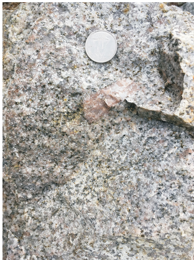
Figure 5: Sample of fresh porphyritic granite of the Tuzo Creek stock; note subhedral K-feldspar phenocryst in a granular quartz, K-feldspar, plagioclase matrix.
