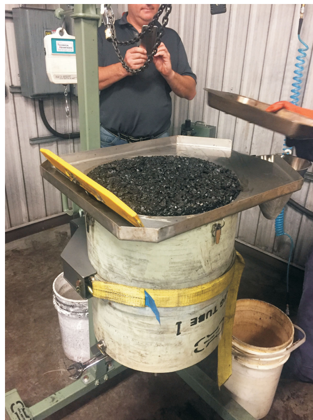
Figure 5. Inverted Roben Jig with coal slice to be removed.
