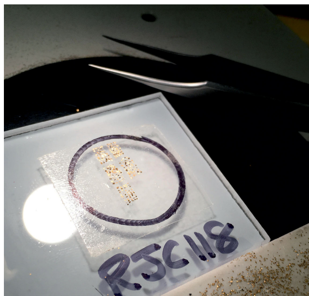
Figure 2. Gold particles are mounted in circular blocks of resin, which are then polished to reveal the particle interiors for analysis.
