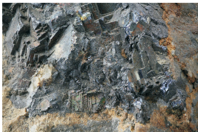
Figure 3. A series of macroscopic images are taken at different locations (focal depth) on the sample and are focus stacked to produce high-resolution images. (Left) Massive sphalerite vein. (Right) High-grade vein material from the Granisle mine, Babine Lake, British Columbia (specimens courtesy of the Smithers Exploration Group).
