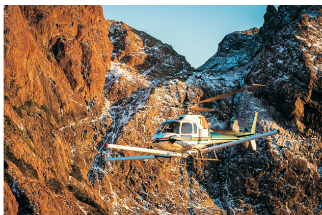
Figure 3. Precision GeoSurveys Inc.'s Airbus AS350 helicopter, which was used to fly the Vancouver Island North airborne survey. Survey equipment included three Scintrex CS-3 cesium-vapour airborne magnetometer sensors arranged into a triple-boom magnetometer configuration (shown), and 21 L of sodium iodide (NaI) gamma radiation detection crystals. Photo courtesy of Precision GeoSurveys Inc.
