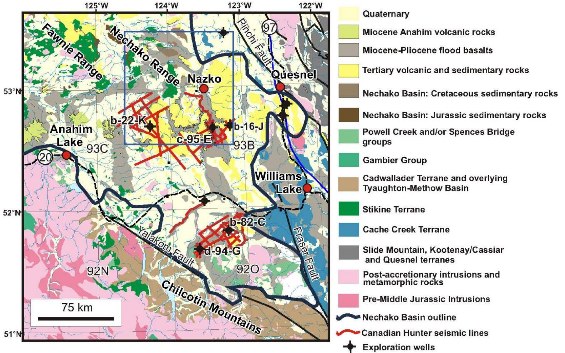
**Figure 1.** Geology of the southern Nechako Basin (outlined by thick purple line), showing locations of industry seismic reflection lines and exploratory drillholes. The blue rectangle identifies the area of the map in Figure 2. Numbers of 1:250 000 NTS map areas are indicated. Map provided by F. Ferri, BC Ministry of Energy, Mines and Petroleum Resources.
