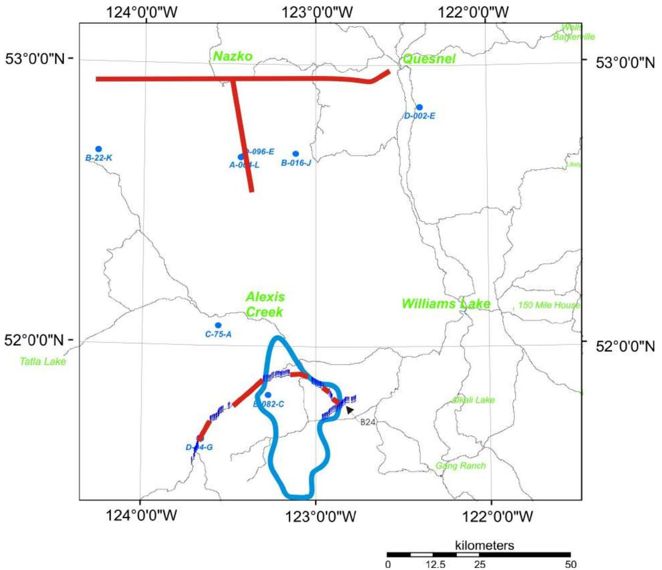
**Figure 2.** Locations of the MT profiles (thick orange lines) along which data is expected to be collected by the end of November 2007. The blue exclamation points show the locations of the sites collected to date, and the light blue line marks the outline of the observed gravity low. The light blue circles show borehole names and locations.
