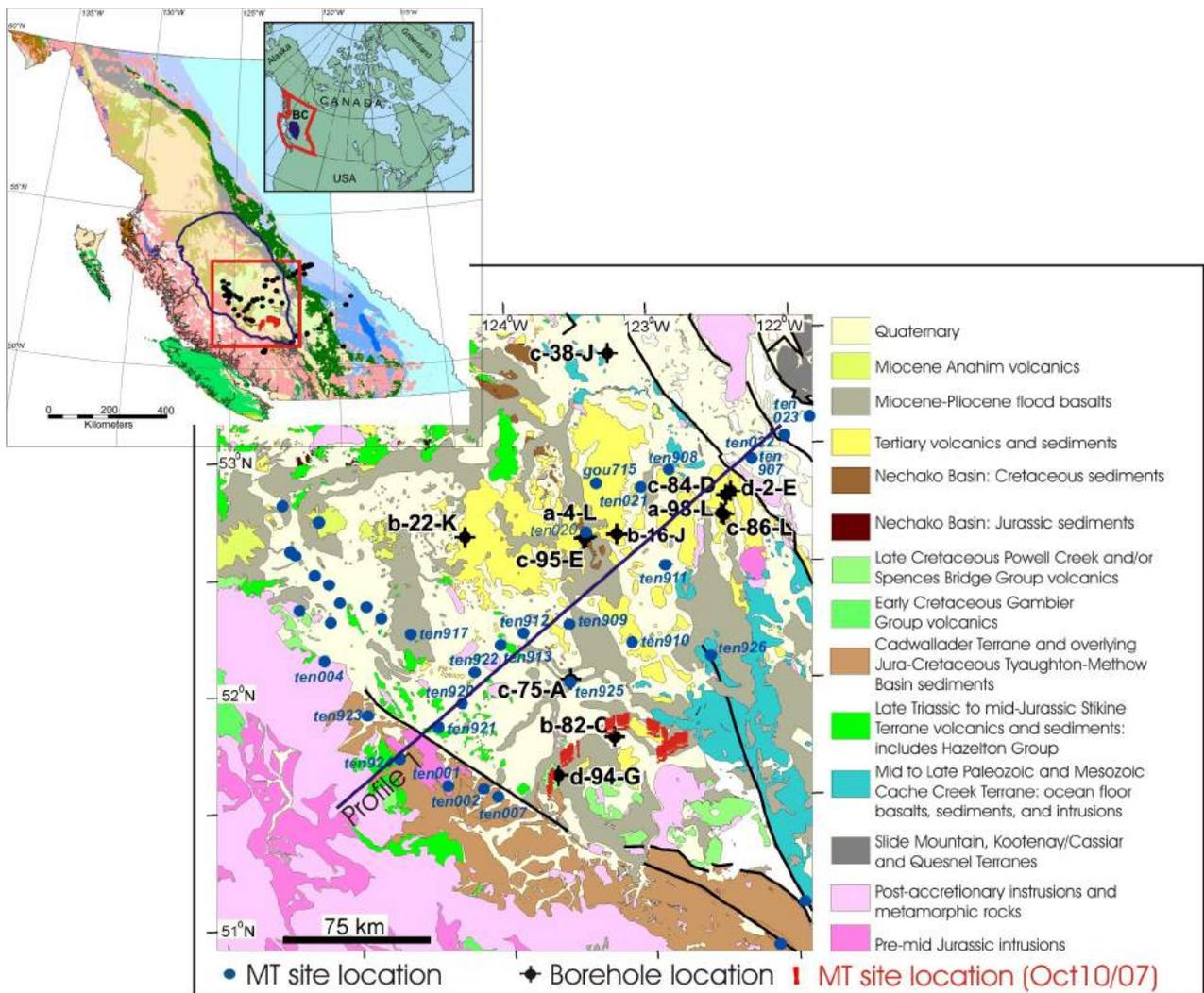
**Figure 1.** Location and geology of the Nechako Basin, showing the locations of the boreholes, old MT sites and the newly acquired MT sites. The blue outline on the location map in the upper left shows the outline and extent of the Nechako Basin. The blue line labelled 'Profile 1' is the surface trace of the two-dimensional model shown in Figure 3.
