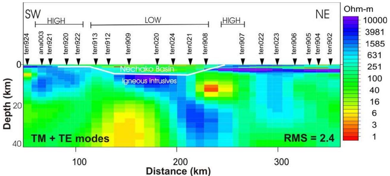
**Figure 3.** Two-dimensional conductivity model from 20-year-old MT data that were re-analyzed using modern techniques. The red and blue colours represent conductive and resistive regions, respectively. The white line (from Spratt et al., 2006) marks the interpreted boundary of the Nechako Basin.
