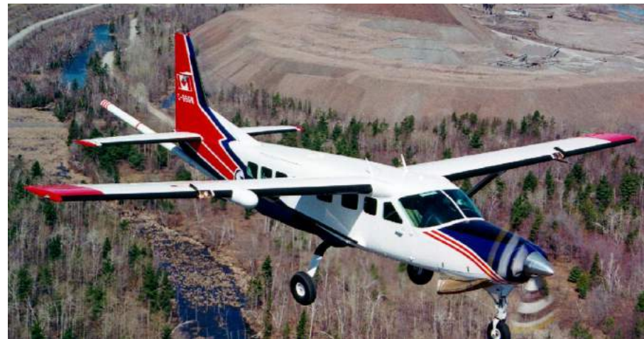
Airplane flying an airborne gravity survey, which measures the density of rocks. All survey equipment is contained within the airplane. The airplane will operate out of local airports. Photo courtesy of Sander Geophysics Ltd.
