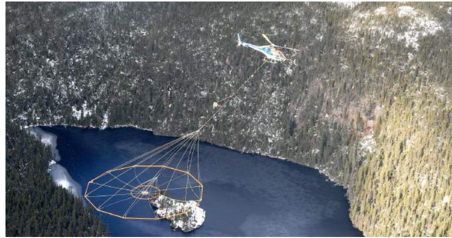
Helicopter flying airborne electromagnetic geophysical survey (survey equipment, which looks like a giant spiderweb, is suspended beneath the helicopter). Geophysics is essentially remote sensing of the properties of rocks in the ground, in this case being the conductivity of the rocks. The helicopter will operate out of airports, roads, and open areas where it can land for re-fueling.
