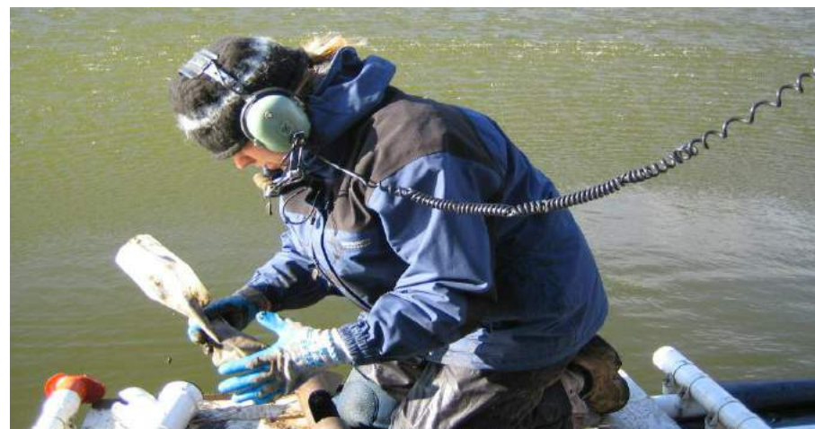
Sampling of lake sediment for geochemical analysis. Geochemistry involves the sampling of sediment from lakes and streams, looking for unusual concentrations of elements of interest such as copper or gold. Sampling crews will work from trucks and helicopter. This new geochemical data will identify new potential mineral exploration targets, and help attract the exploration industry to the region.
