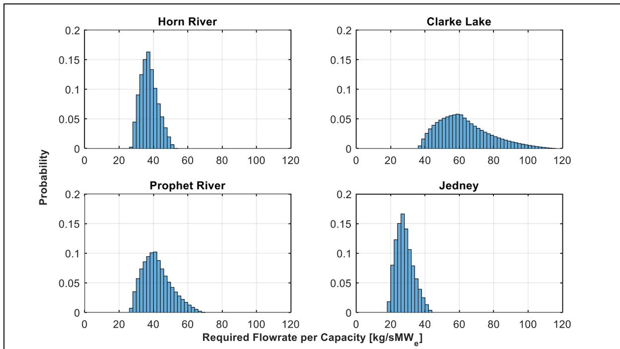
Figure 18 Probabilities of required brine flow rate per megawatt of installed electric capacity
