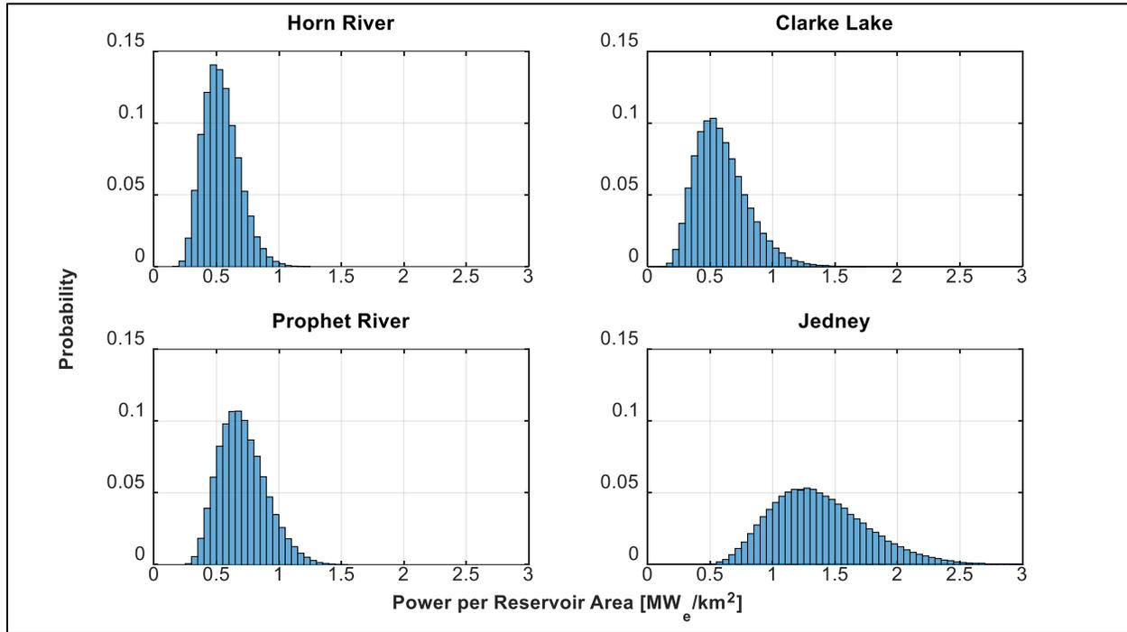
Figure 17 Probabilities of potential electric power output per unit reservoir area
