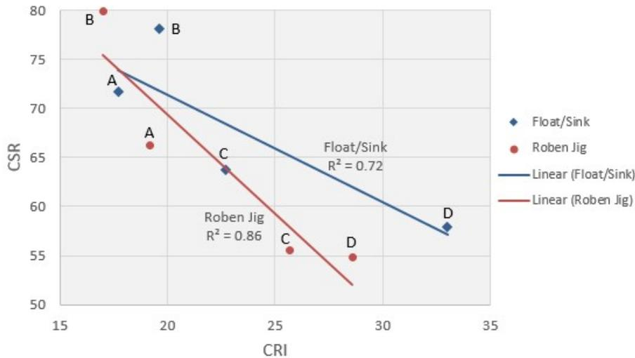
Figure 9. Plot showing CSR and CRI data for all four coal types.
