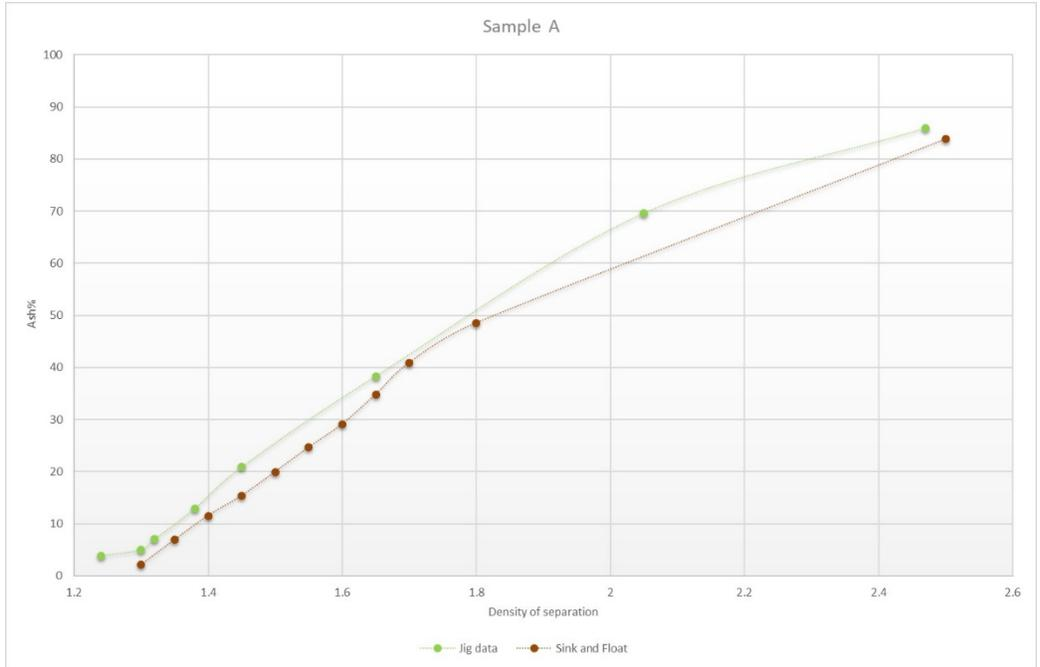
Figure 10b. Density of separation (S.G. and ARD) vs. ash in density fractions for sample A.
