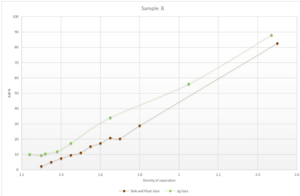
Figure 11b. Density of separation (S.G. and ARD) vs. ash in density fractions for sample B.
