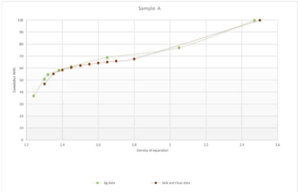
Figure 10c. Density of separation vs. cumulative yield of clean coal for sink and float and jig procedures.
