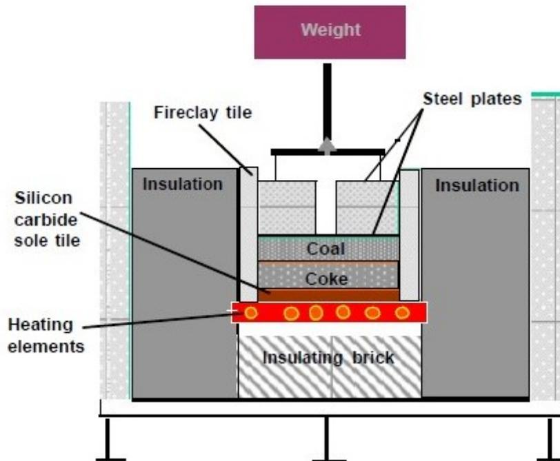
Figure 6 – Schematic diagram of the Sole-Heated Oven.
