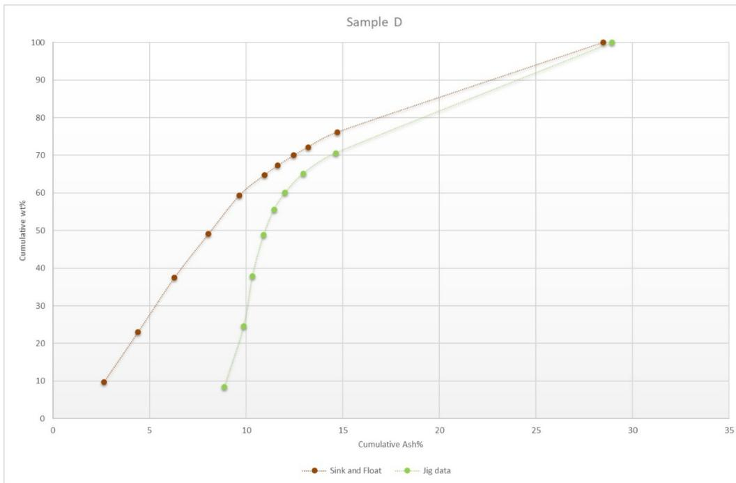
Figure 13a. Clean coal curve for sample D.
