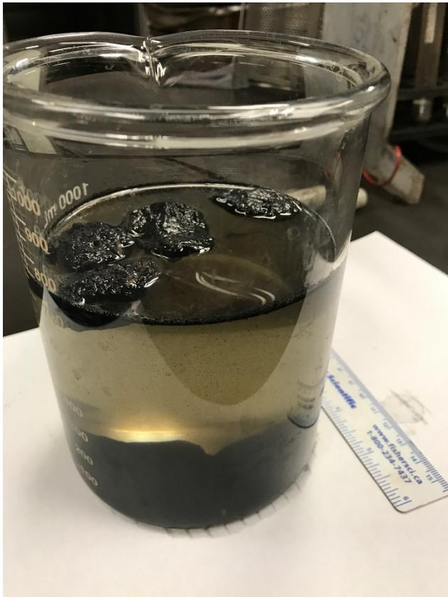
Figure 3. Coal particles floating in perchloroethylene.
