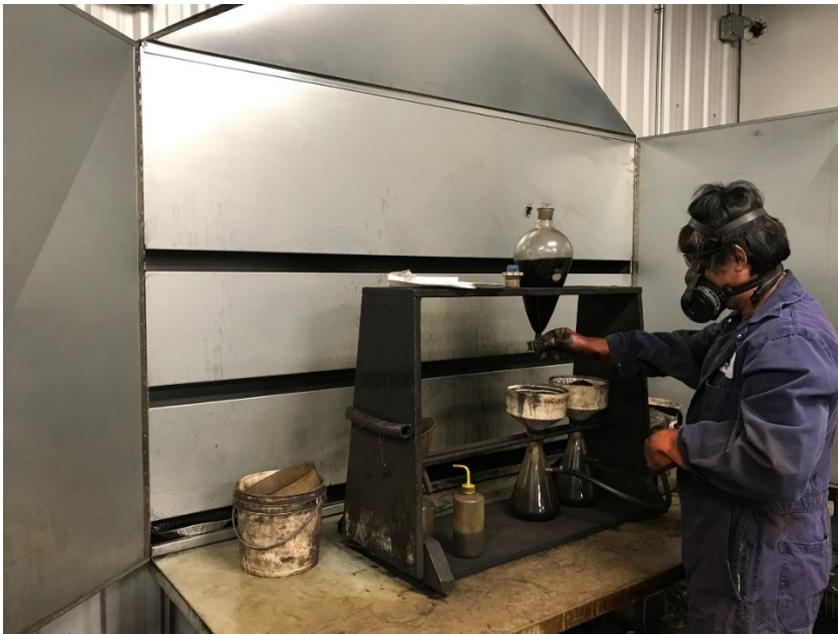
Figure 1. Operator working with organic liquids in a specially designed fume hood.
