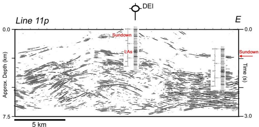
**Figure 4.** Portion of seismic line 11p with the synthetic seismic trace from the DEI drill hole spliced into the data. Two splices are shown: the one labeled ‘DEI’ is at the location of the drill hole; the one on the right side of the section projects the drill hole down dip to the east to illustrate the consistent reflection character (sundown reflection – quiet zone near LMc- strong LAs reflections). ‘LAs’ = lower Aldridge sills (probably partly equivalent to the Bootleg sills).
