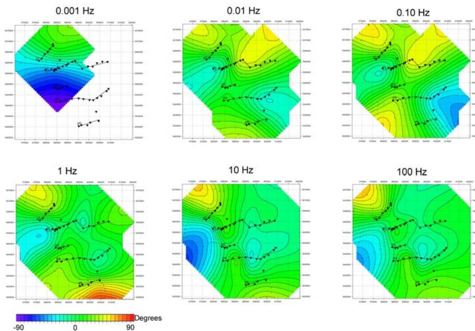
**Figure 5a.** Maps of the impedance strike for lines P1 (north) through P5 (south) and for different frequencies.
