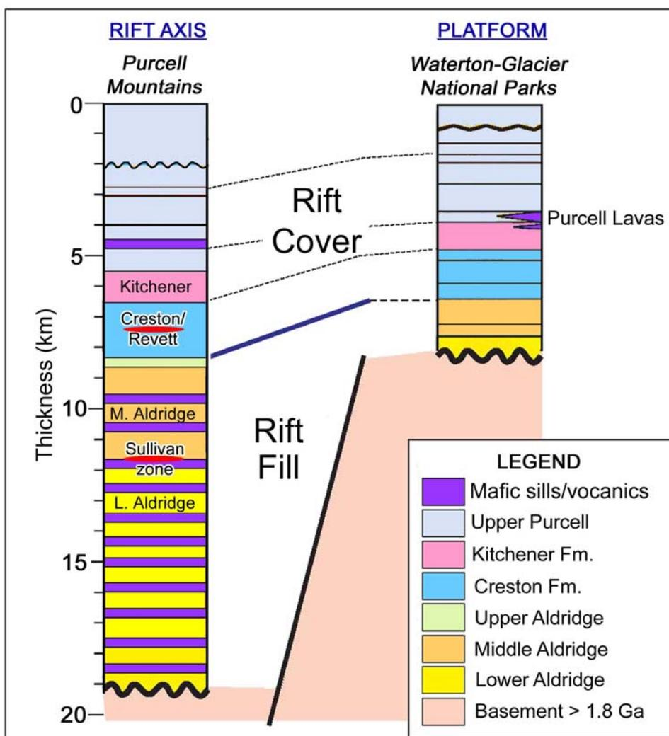
**Figure 2.** Stratigraphic cross section from the Waterton/Glacier park area on the east to the center of the Purcell anticlinorium in the vicinity of the Moyie anticline on the west (modified from Lydon, 2007). The rocks of greatest interest for this study are the Aldridge, Creston and Kitchener formations. The stratigraphic position of the Sullivan sedex deposit is shown as ‘Sullivan zone’.
