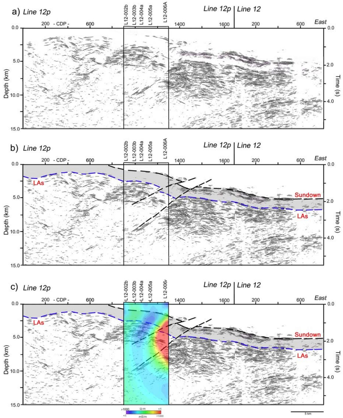
**Figure 13.** a) Uninterpreted seismic line 12 (12p-12) with the locations of the MT stations for MT liner P3 indicated; b) Interpretation of the Middle Aldridge Sundown (black line) to Lower Aldridge sills (LAs, blue line) interval indicated in gray. The Lower-Middle Aldridge transition (‘Sullivan horizon’) is located within the Sundown-LAs interval; c) Same as (b) with the MT inversion of line P3 overlain. Note the high conductivity indicated near the interpreted faults.
