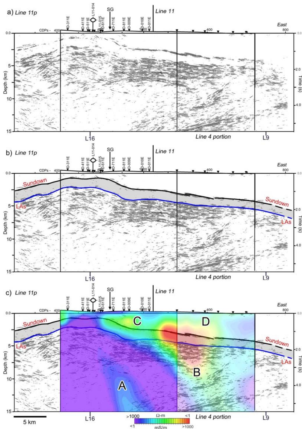
**Figure 18.** a) Uninterpreted seismic line 11 (combined lines 11p-11); b) Interpretation of the Middle Aldridge Sundown (black line) to Lower Aldridge sills (LAs, top indicated with blue line) indicated in gray. The Lower-Middle Aldridge transition (“Sullivan horizon”) is located within the Sundown-LAs interval; c) Same as (b) with the MT inversion of line P2 overlain. Note that the high conductivity (red) is in a similar stratigraphic position as the high conductivity of zone 2 in Figure 17c.
