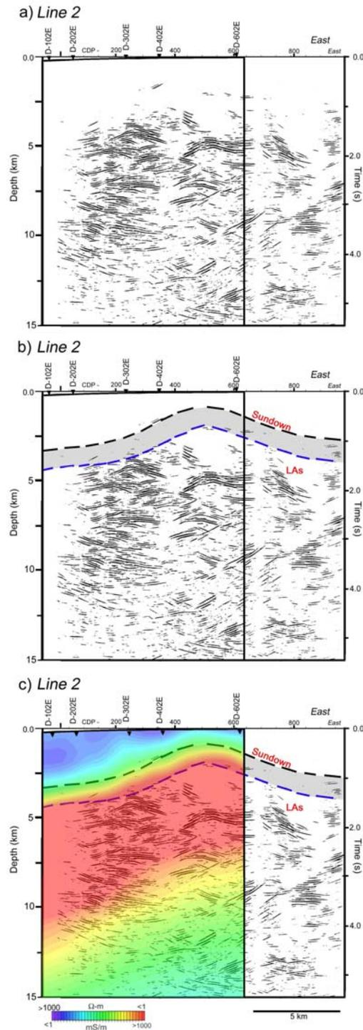
**Figure 12.** a) Uninterpreted seismic line 2 with the locations of the MT stations indicated; b) b) Interpretation of the Middle Aldridge Sundown (black line) to Lower Aldridge sills (LAs, top indicated with blue line) indicated in gray. The Lower-Middle Aldridge transition (“Sullivan horizon”) is located within the Sundown-LAs interval; c) Same as (b) with the MT inversion of line P5 overlain. Note that the high conductivity extends to ~12 km depth (about 7-8 km beneath the top of LAs).
