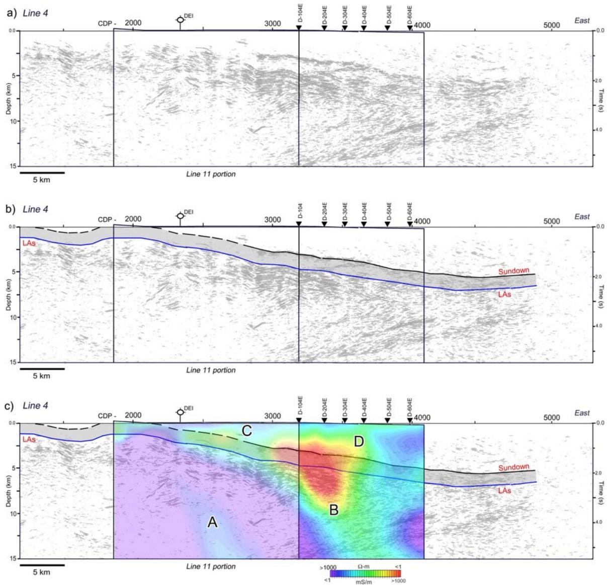
**Figure 18.** a) Uninterpreted seismic line 4; b) Interpretation of the Middle Aldridge Sundown (black line) to Lower Aldridge sills (LAs, top indicated with blue line) indicated in gray. The Lower-Middle Aldridge transition (“Sullivan horizon”) is located within the Sundown-LAs interval; c) Same as (b) with the MT inversion of line P3 overlain. Note that the highest conductivity (red) is in a similar stratigraphic position as the high conductivity along line 12-P4 (Figure 17c).
