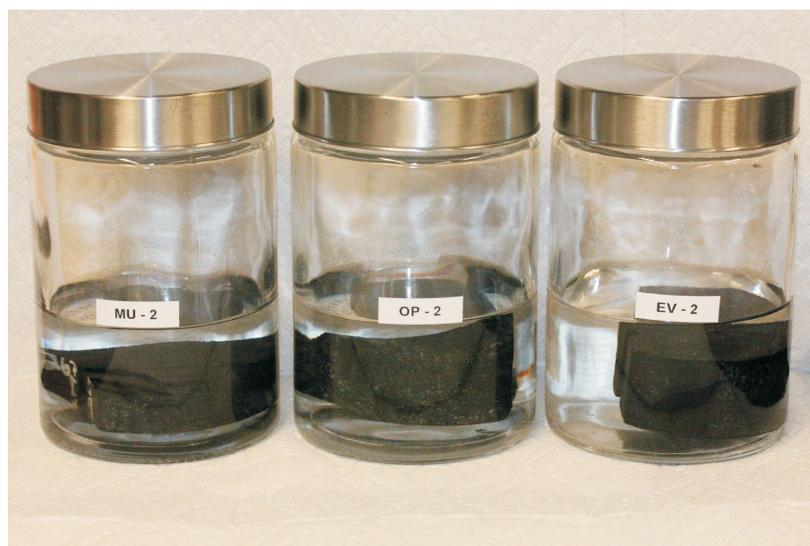
**Figure 3:** Imbibition cells used in phase 1. Rock samples were immersed in aqueous or oleic phases. Change in mass of the rock samples and electrical conductivity of the fluid (for aqueous-phase experiments) were recorded periodically.
