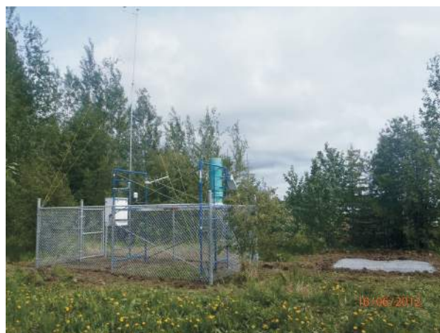
Figure 2. Photograph of Kiwigana River climate station, northeastern British Columbia. The white object on the ground, to the right of the climate station, is a snow pillow. Photo courtesy of B. Ortman, Peace Country Technical Services Ltd.
