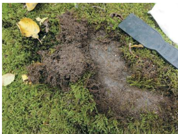
Figure 4. A typical moss-mat sediment sample, British Columbia, 3.8 cm (1.5 in) plastic putty knife for scale.
