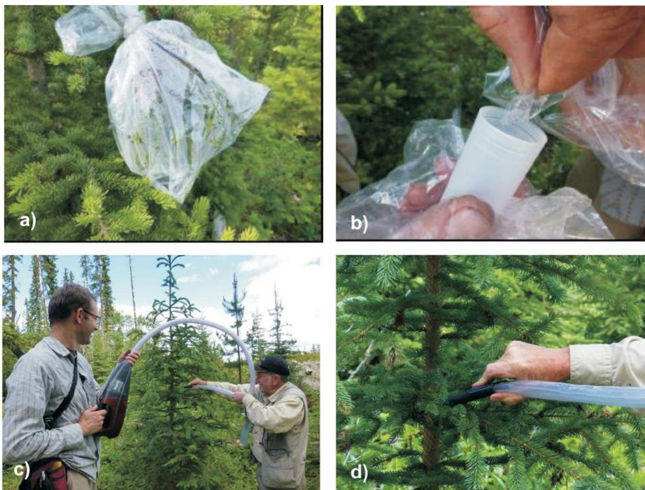
**Figure 8.** Collection of exudate samples at the Woodjam property, south-central British Columbia: **a)** and **b)** transpired fluids; **c)** and **d)** surface particulates, using a vacuum and cyclone system.
