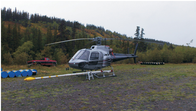
Figure 3. HeliMAG stinger system used by Geo Data Solutions Inc. to fly the Block 2 survey in the Dease Lake and Telegraph Creek areas. Photo courtesy of Geo Data Solutions Inc., Laval, Quebec.
