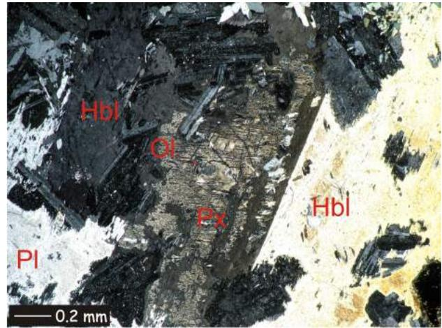
**Figure 11.** Photomicrograph of medium-grained hornblende gabbro from the Norgate Creek area. Olivine altered to serpentine and saussuritized plagioclase are cumulus crystals within intercumulus zones of serpentinized pyroxene with fresh hornblende rims. Low interference colours (crossed polars) are due to thinning of the thin section at its edge.
