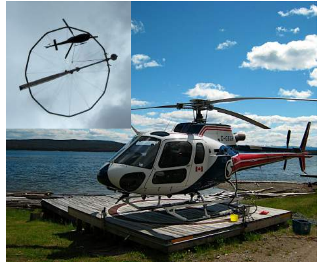
Helicopter used in flying an airborne gravity survey. All survey equipment is contained within the helicopter. Photo courtesy of O. Peterson, Sander Geophysics Ltd.
