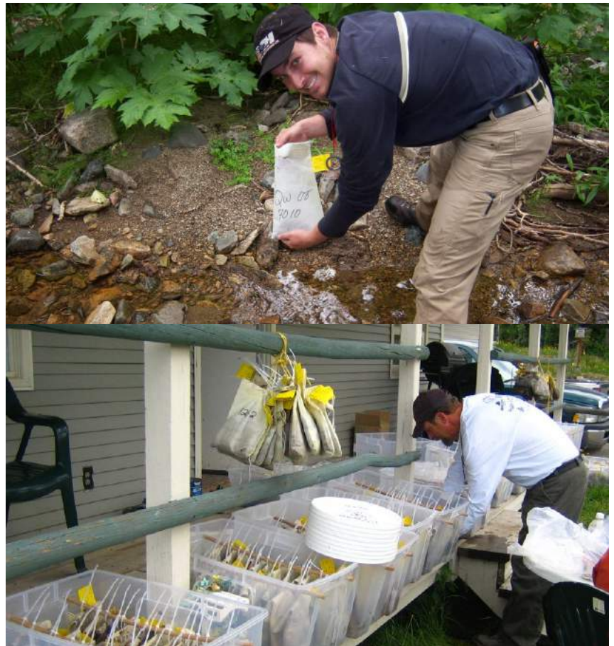
Sampling and storage of stream sediment for geochemical analysis. Photo courtesy of W. Jackaman, Noble Exploration Services Ltd.
