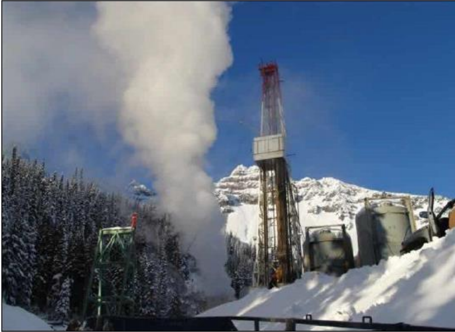
Photo: Flow test of well MC-6 at the South Meager geothermal project (Source: ThinkGeoEnergy website: www.thinkgeoenergy.com )
