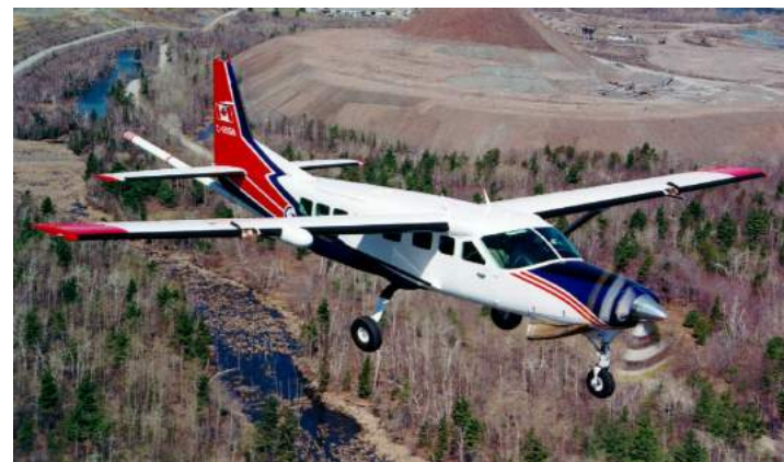
PHOTO 2. Airplane flying an airborne gravity survey. All survey equipment is contained within the airplane. Photo courtesy of Sander Geophysics Ltd.
