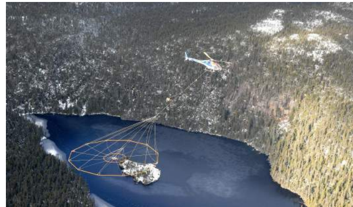
PHOTO 1. Helicopter flying airborne electromagnetic survey. The electromagnetic survey equipment is suspended beneath the helicopter. Photo courtesy of Geotech Ltd.
